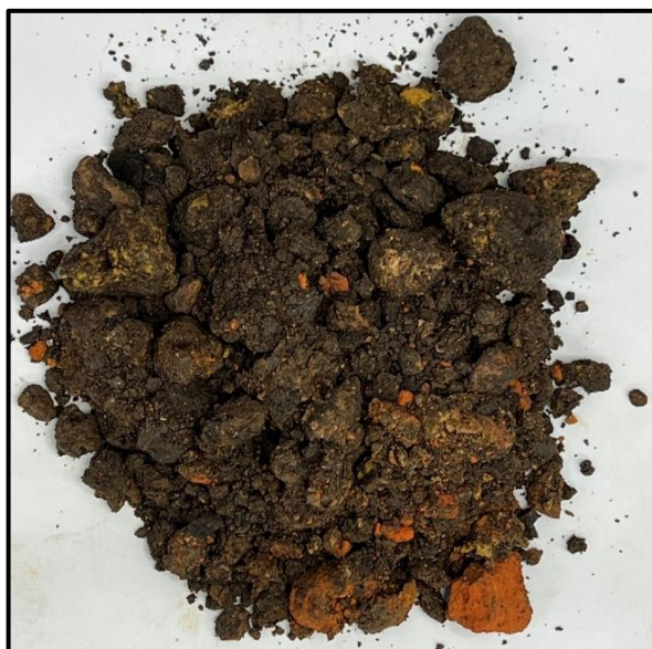
Figure 3: (Left) Stratum II CH material from B-06 approximately 2.0 feet below the existing surface elevation.
