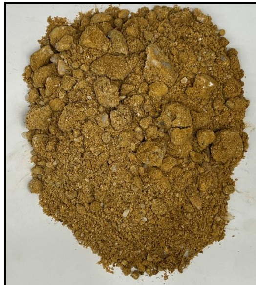
Figure 7: (Left) Stratum III GC material from B-01 approximately 8.5 feet below the existing surface elevation.
