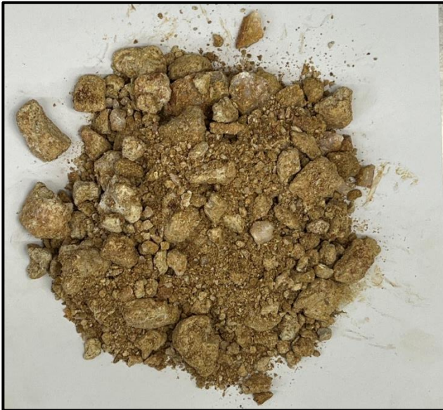
Figure 7: (Left) Stratum III GC material from B-01 approximately 8.5 feet below the existing surface elevation.
