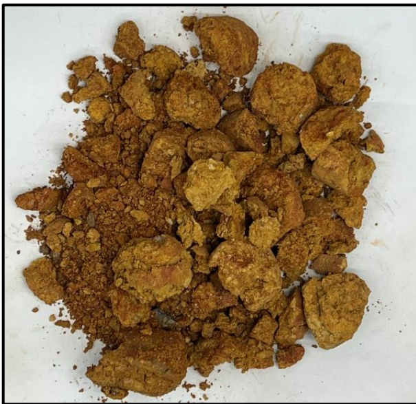
Figure 3: (Left) Stratum II CH material from B-06 approximately 2.0 feet below the existing surface elevation.
