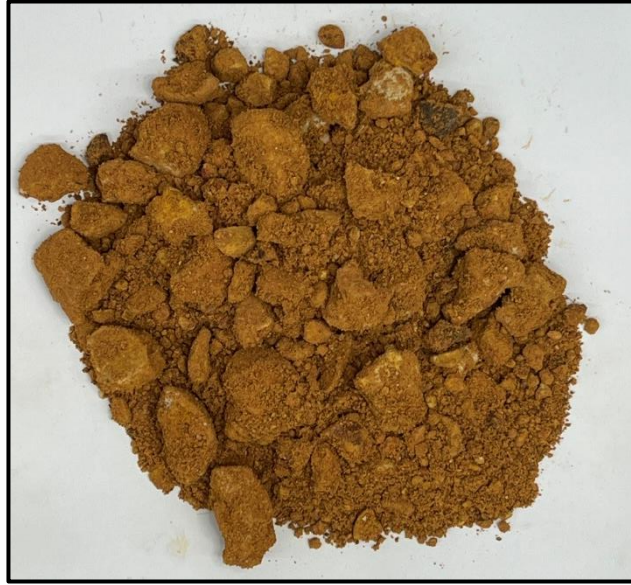
Figure 5: (Left) Stratum III SM material from B-04 approximately 3.5 feet below the existing surface elevation.
