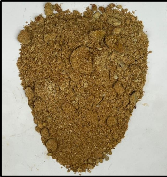
Figure 5: (Left) Stratum III SM material from B-04 approximately 3.5 feet below the existing surface elevation.
