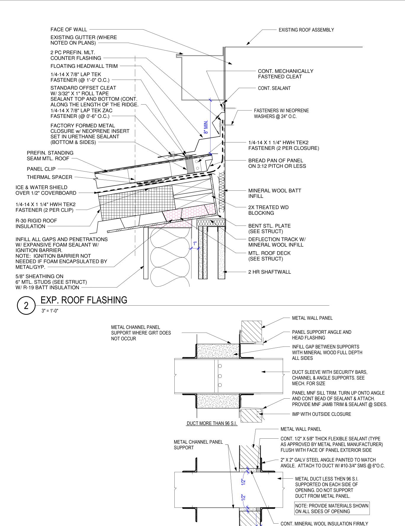
EXTERIOR WALL DUCT PENETRATION- NON RATED
