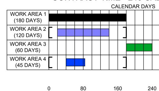
BRACKETED PHASES INDICATE THAT THE WORK WITHIN THIS PHASE CAN BE COMPLETED AT ANY DATE WITHIN THE BRACKETS SHOWN AS LONG AS IT IS COORDINATED WITH THE RPR BEFORE PHASED WORK BEGINS.
