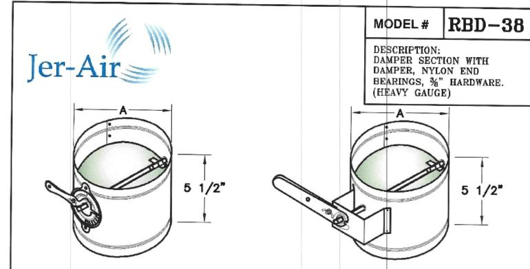
A HEAVY DUTY MANUAL BALANCING DAMPER WHICH MEETS OR EXCEEDS SMACNA STANDARDS AS PER HVAC DUCT CONSTRUCTION STANDARDS - SECOND EDITION - 1995
