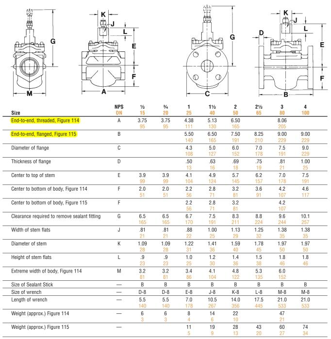
Flanges are drilled to ANSI Class 125 Cast Iron Flange Standard Template. For drilling and bolting data, See page 40.
