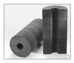
With the patented StrataFab® System, blocks of FOAMGLAS® insulation are laminated into billets using a special high temperature adhesive. These billets are fabricated into the desired shapes and sizes for pipe, tank, vessels, flanges and valves—practically any industrial insulation application.
