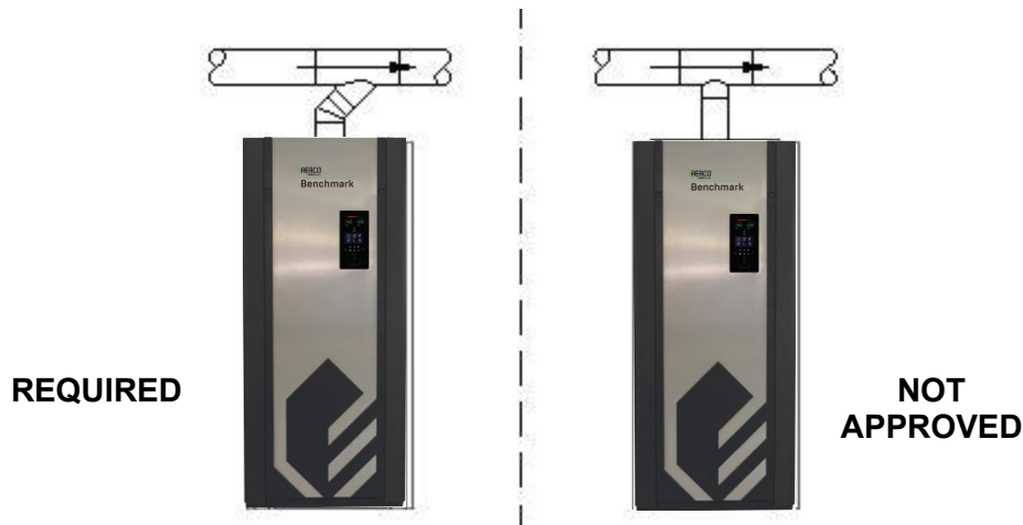
Figure 11a: Required Connections to Common Vent Breeching
