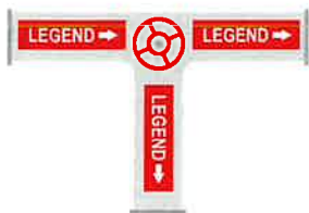
Adjacent To Valves & Flanges
