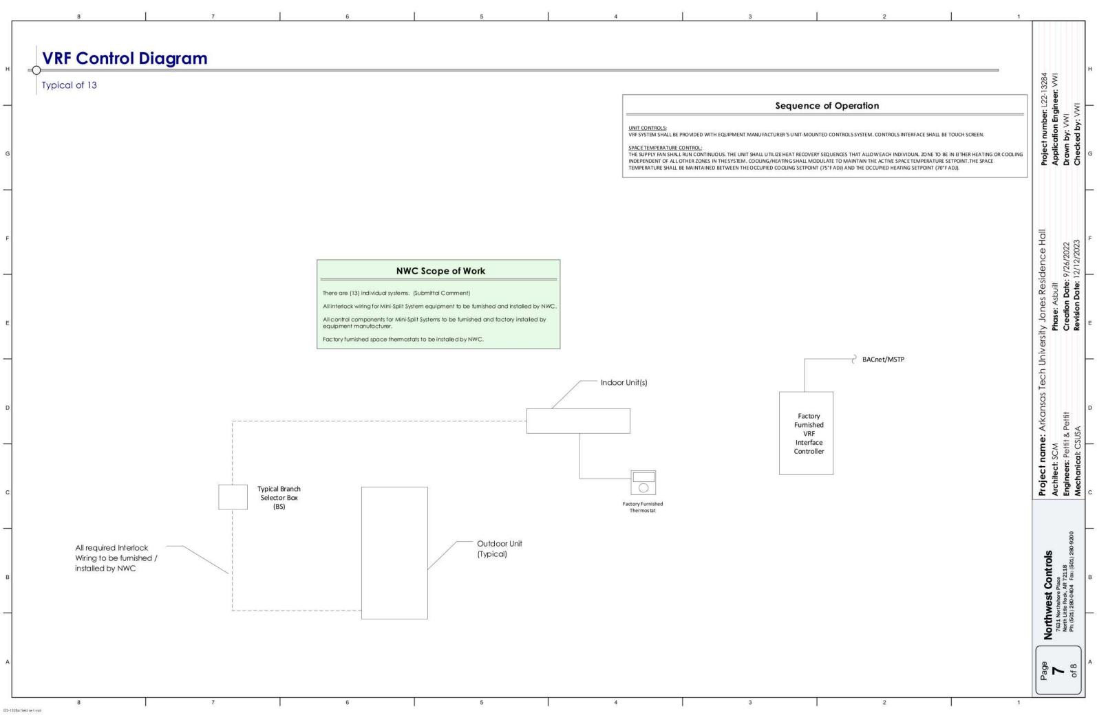
All controller inputs, outputs and communications trunks must be run separate from any circuits containing voltages greater than 30 vac.
