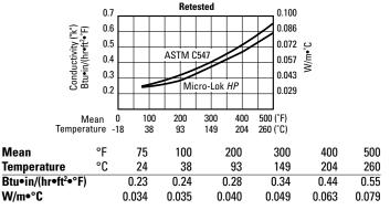
\* Apparent thermal conductivity values are determined by applying procedures dictated per ASTM C1045 on test data obtained using ASTM Test Method C335. All values are based on nominal manufacturing and testing parameters, are subject to normal variation, and are not guaranteed for specification purposes or otherwise.
