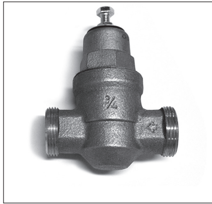
A Pressure Reducing Valve is required if your home's water pressure is above 80 psi.
