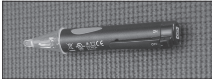
Figure 2 - Use a non-contact circuit tester to insure that the power is off before you work on a circuit.
