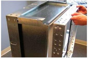
**STEP 6:** Place a latch so that the 2 tabs of the latch overlap the prefilter frame on each side of the corner. Slide the latch inside of the leg extension and align the latches' cap screw with the threaded coupling on the end of the leg extension and tighten using the hexkey. See Figure 43.
