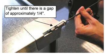
**STEP 4:** Once all four corner latches have been tightened within 1/4" of the leg extension coupling, complete the installation by tightening each corner until the latch and leg extension coupling meet. This is illustrated in Figure 26.
