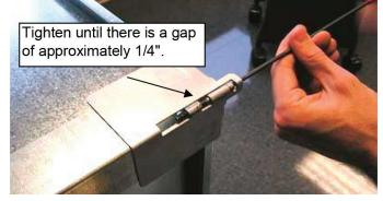
**STEP 4:** Once all four corner latches have been tightened within 1/4" of the leg extension coupling, complete the installation by tightening each corner until the latch and leg extension coupling meet. This is illustrated in Figure 40.
