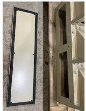
Figure 90: Side flange to be secured once side panel is removed
