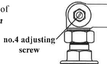
Bottom view of faucet body and Built-in Stop
