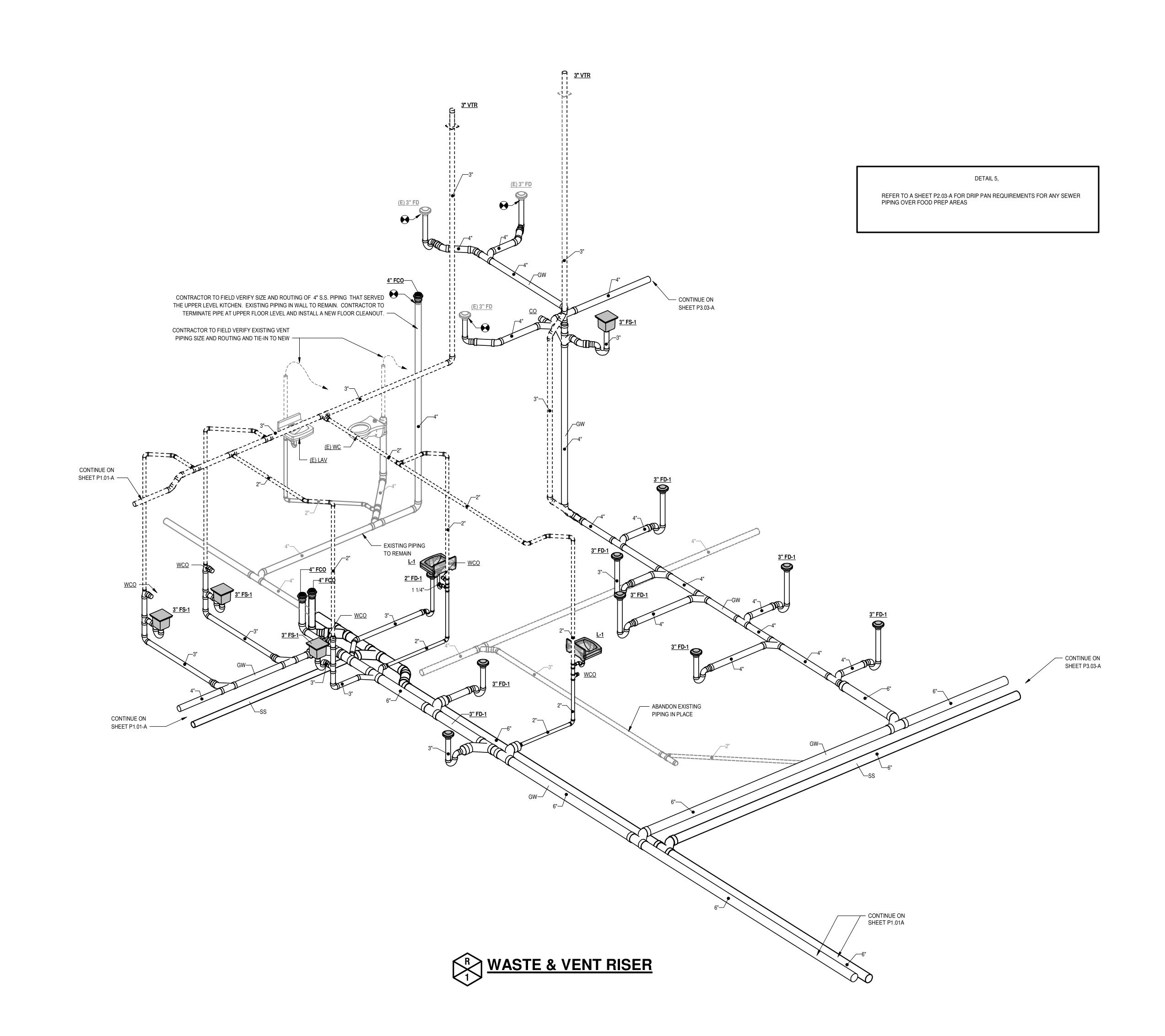
NOTE: ALL FLOOR DRAINS SHALL HAVE TRAP PRIMERS. LOCATE TRAP PRIMER DEVICES IN MECH. ROOMS AND JAN. CLOSETS (IN FINISHED AREAS PROVIDE TRAP PRIMER IN WALL WITH ACCESS PANELS) - FIELD VERIFY EXACT LOCATIONS AND WATER PIPE ROUTING.
