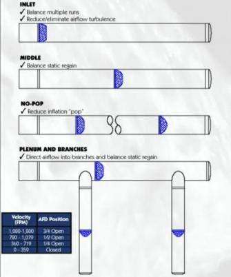
Designed for retrofits as well as new systems, the AFD is easily installed or replaced for laundering in minutes by zipping or unzipping its collar between duct lengths. Besides airflow regulation, the AFD also serves as a flow straightener.
