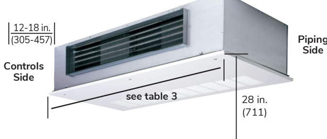
Figure 7. CBY Unit Clearance and Service Access
