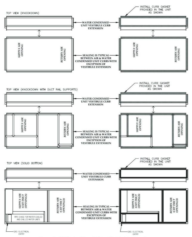
Figure 5 - RN Series 6-8 and 10 ton Unit Isolator Locations
