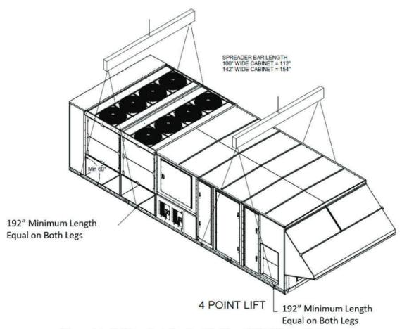
Figure 14 - Lifting Details of a 55, 65 and 75-140 ton Unit
