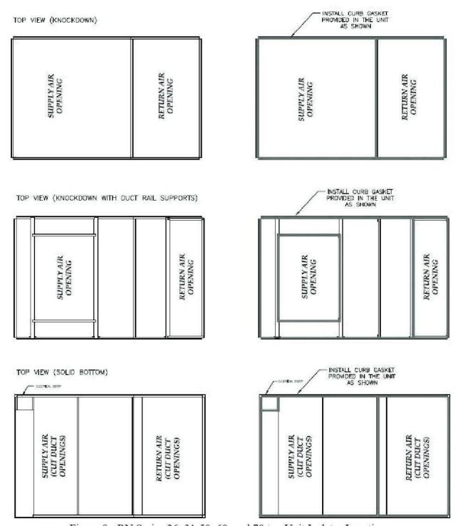
Figure 8 - RN Series 26, 31-50, 60, and 70 ton Unit Isolator Locations
