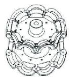
Top half is the HUB. Bottom half is the RET or retainer ring.
