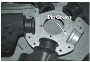
Figure 38 - Pin Groove Location
