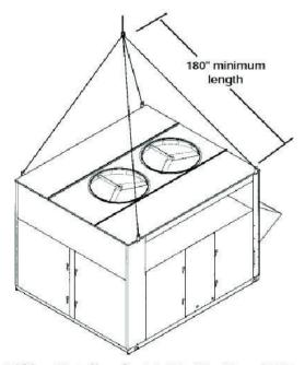
Figure 13 - Lifting Details of a 26, 31-50, 60 and 70 ton Unit
