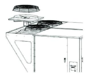
Figure 46 - Removal of a Condenser Fan Assembly
