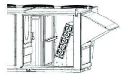
Figure 45 - Evaporator Coil Access
