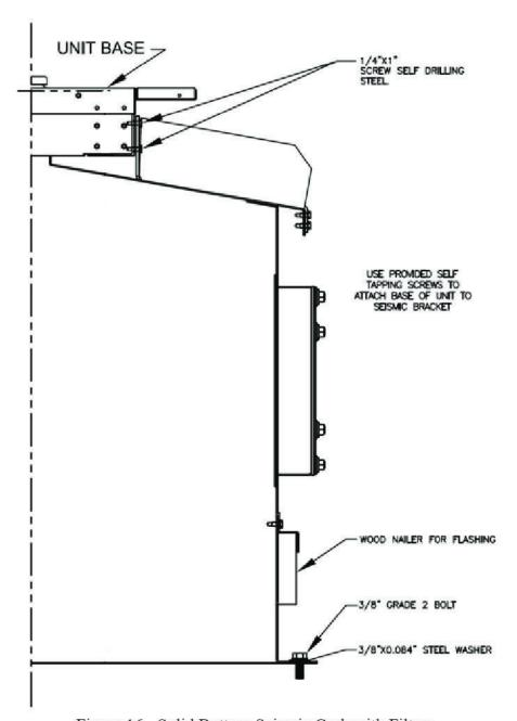
Figure 16 - Solid Bottom Seismic Curb with Filters
