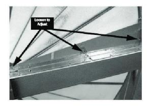
Loosen the three purge adjusting screws. 2. Adjust purge sector to the specified angle.
