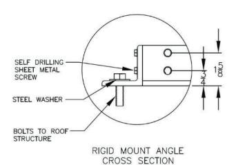
Figure 20 - Seismic Rigid Mount Curb
