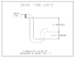
Figure 29 - Draw-Through Drain Trap
