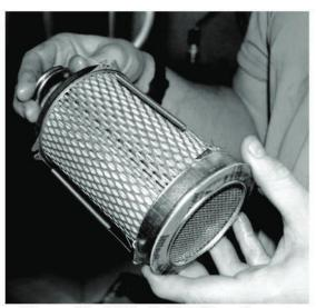
Figure 47 - RPE-48-BD filter element
