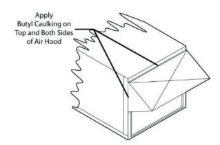
Figure 23 - 26 and 31-140 ton Open Rain Hood
