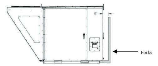
Figure 10 - Forklifting an RN Series A, B and C Cabinet, 6-25 and 30 tons
