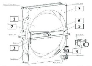
Figure 48 - Aluminum Energy Recovery Wheel
