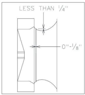
Figure 31 - Plenum Fan Gap Tolerances
