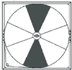
Figure 51 - Wheel Segment Removal Pattern
