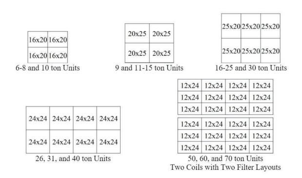
Figure 60 - RN Series 6-50, 60, and 70 ton Standard Filter Layouts
