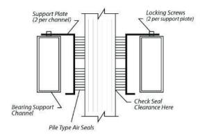
Cross Section of Air Seal Structure
