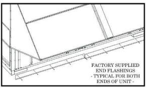
Figure 24 - Factory Supplied End Flashings
