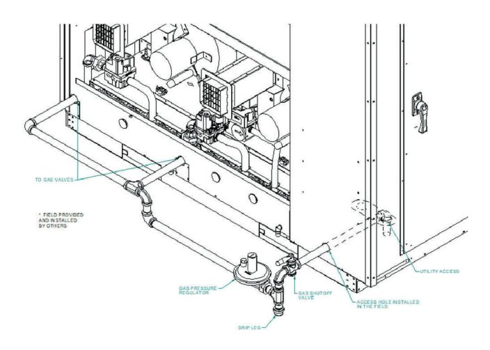
Figure 56 - Example 6-50, 60 & 70 ton External Gas Piping
