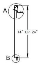
Figure 17 - Seismic Solid Bottom Curb without Filters Cross Section
