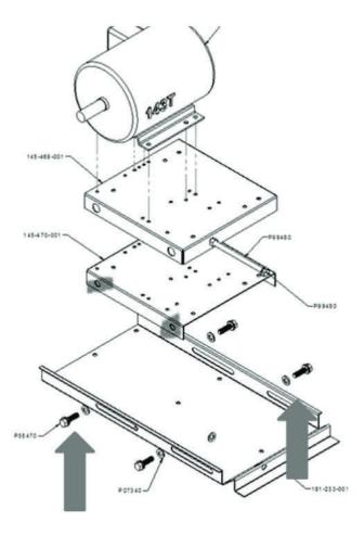
Remove the belt tensioner bolt completely, as indicated by the arrow below.
