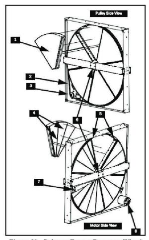
Figure 50 - Polymer Energy Recovery Wheel
