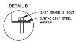
Figure 19 - Seismic Solid Bottom Curb without Filters Detail B
