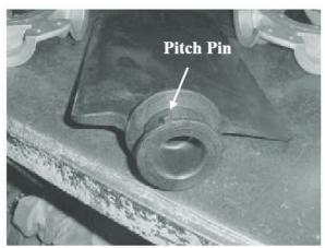
Figure 39 - Pitch Pin Location
