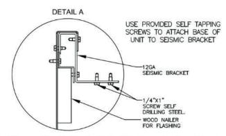
Figure 18 - Seismic Solid Bottom Curb without Filters Detail A
