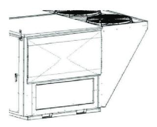
Figure 21 - 6-25 and 30 ton Closed Rain Hood
