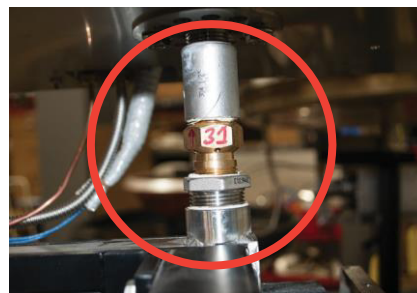
Figure 9.1 – Locating orifice for cleaning
