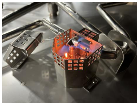
Figure 9.2 – Pilot flame coverage of thermocouple.
