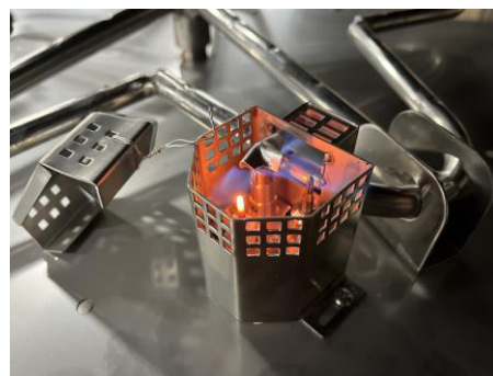
Figure 9.2 – Pilot flame coverage of thermocouple.
