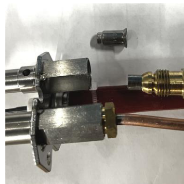
Figure 9.3 – Cleaning pilot orifice
