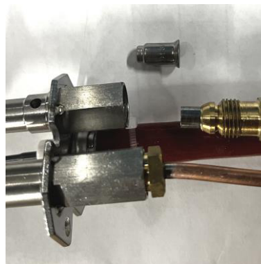
Figure 9.3 – Cleaning pilot orifice
