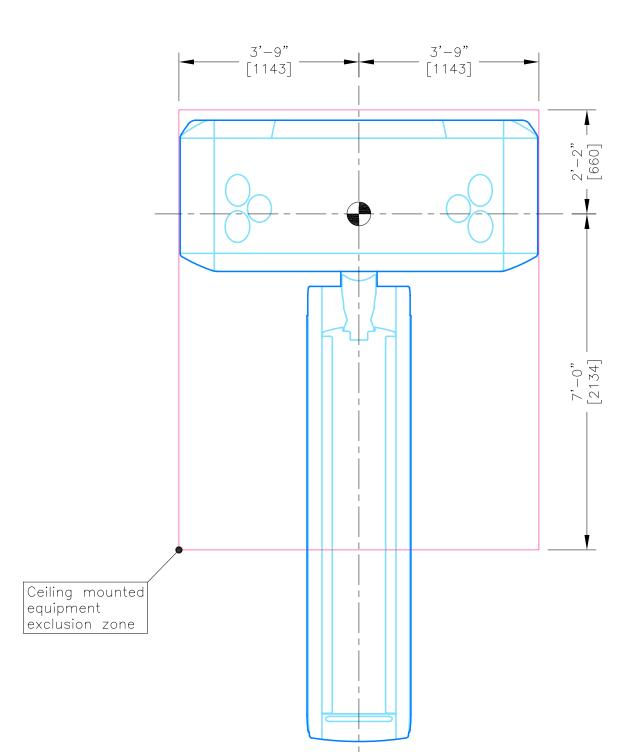
A. Ceiling mounted equipment must be positioned to avoid interference with gantry.
