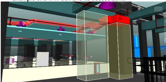
Example of a VAV box and its access zone.
