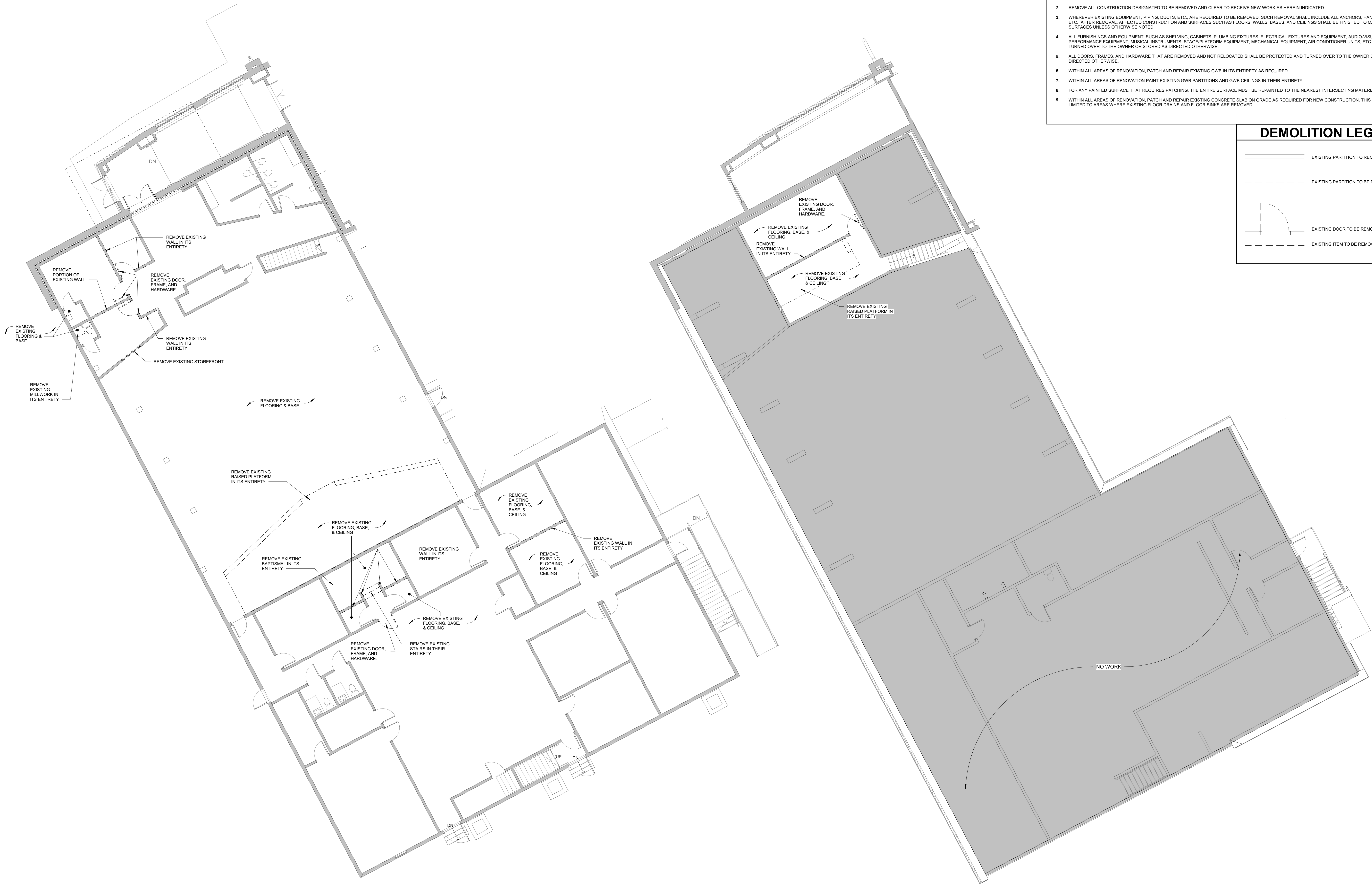
1 FIRST FLOOR DEMOLITION PLAN. 1/8" = 1'-0"
