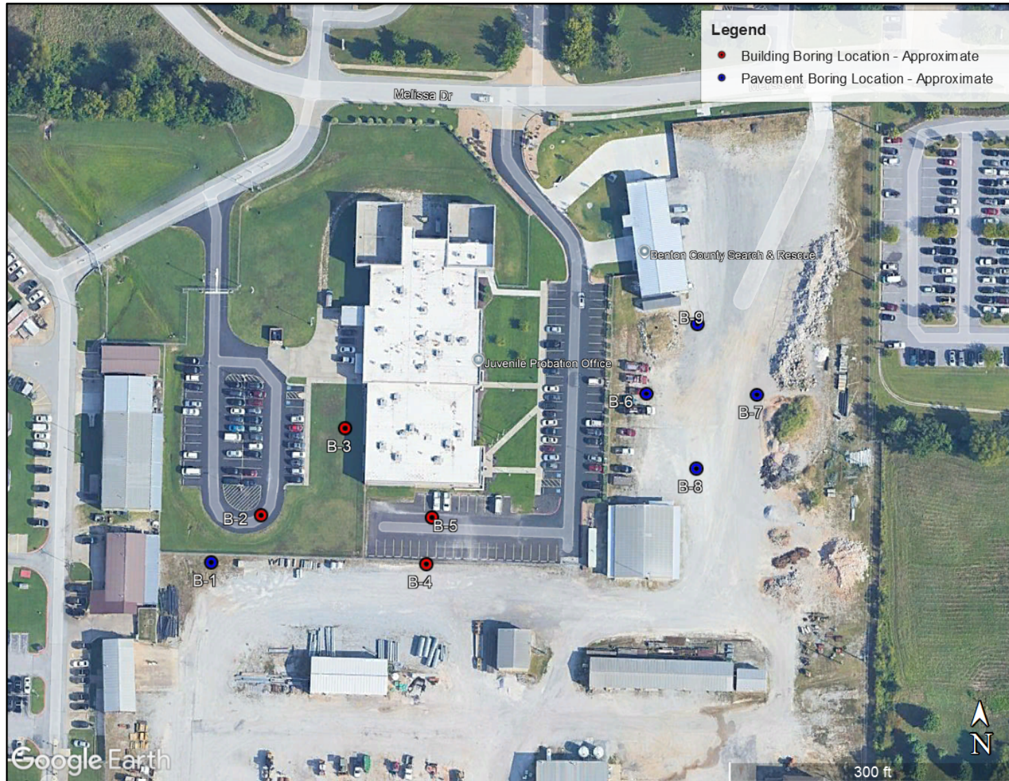
Boring Location Diagram – Aerial Imagery Taken 9/13/2019
