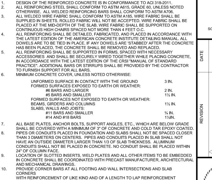
ACCORDING TO TABLE BELOW. 11. ALL LAP SPLICES SHALL BE IN ACCORDANCE WITH THE FOLLOWING TABLE, UNLESS
