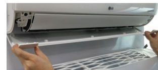
Figure 98: Checking that All Attachment Locations Are Secure (Step 5).
