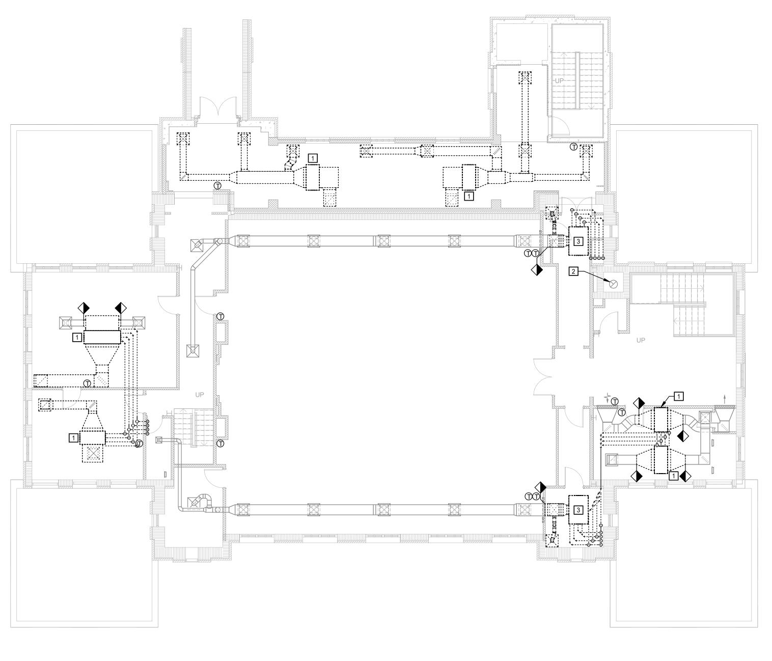
THIRD FLOOR DEMOLITION PLAN - HVAC SCALE: 1/8" = 1'-0"
