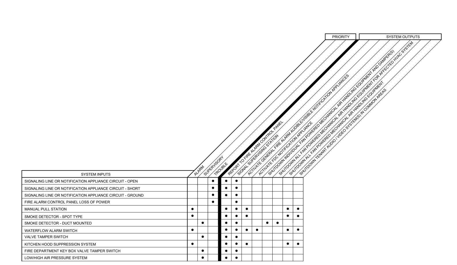
EXISTING SEQUENCE OF OPERATION TO REMAIN. REFER HERE WHERE GUIDANCE IS NEEDED. CONTRACTOR TO PROVIDE ALL NECESSARY EQUIPMENT AND CONNECTIONS REQUIRED TO ACCOMPLISH THE FUNCTIONS INDICATED, AT MINIMUM. SEQUENCE OF OPERATIONS INDICATED IS SCHEMATIC. MODIFY TO SUIT CONDITIONS AND MEET APPLICABLE CODE REQUIREMENTS.
