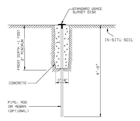
8. At a minimum new benchmarks shall be set as follows: 8" Diameter concrete collar, 24" deep, with a 5/8" rebar approximately 4' long, and a brass cap set on the rebar.
