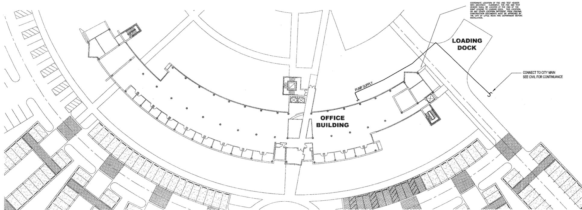
COORDINATE LOCATION OF FDC AND TEST HEADERS WITH ARCHITECT. CURRENTLY, THE FDC AND TEST HEADERS SHALL BE LOCATED AT THE END OF THE RAMP LEADING TO LOADING DOCK. THIS LOCATION OF ANY OTHER LOCATION DIFFERENT FROM ORIGINAL CONSTRUCTION DOCUMENTS MUST BE APPROVED BY THE CITY OF LITTLE ROCK FIRE DEPARTMENT BEFORE INSTALLATION.
