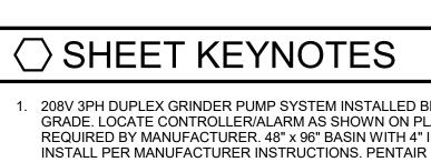
1. 208V 3PH DUPLEX GRINDER PUMP SYSTEM INSTALLED BELOW GRADE. LOCATE CONTROLLER/ALARM AS SHOWN ON PLANS OR AS REQUIRED BY MANUFACTURER. 48" x 96" BASIN WITH 4" INLET. INSTALL PER MANUFACTURER INSTRUCTIONS. PENTAIR MYERS VS50 WITH 5HP PUMP, #VS50-03, OR EQUIVALENT. VERIFY PUMP SIZING WITH MANUFACTURER.
