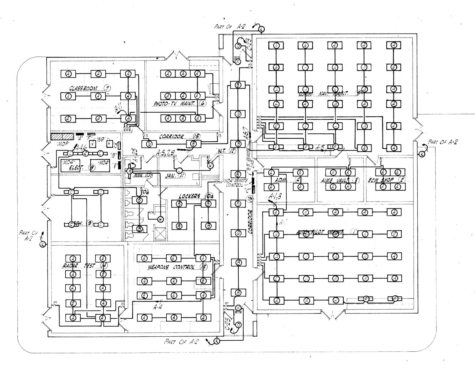
NOTE: Fixtures "E" & "G" are furnished w/battery operated emergency lts. for egress in case of power failure.
