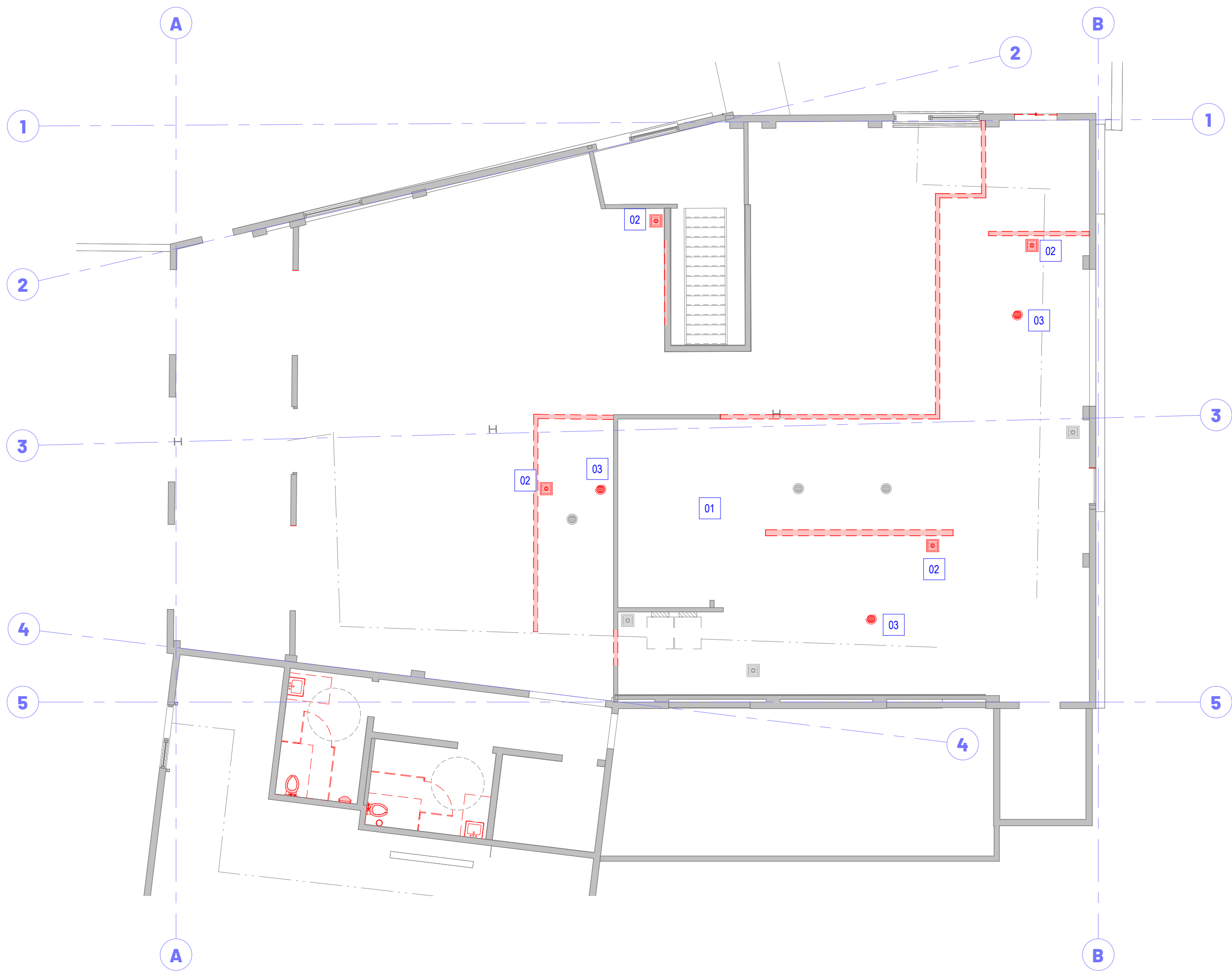
A SLAB DEMO PLAN 1/8" = 1'-0" 0' 4' 8' 16'
