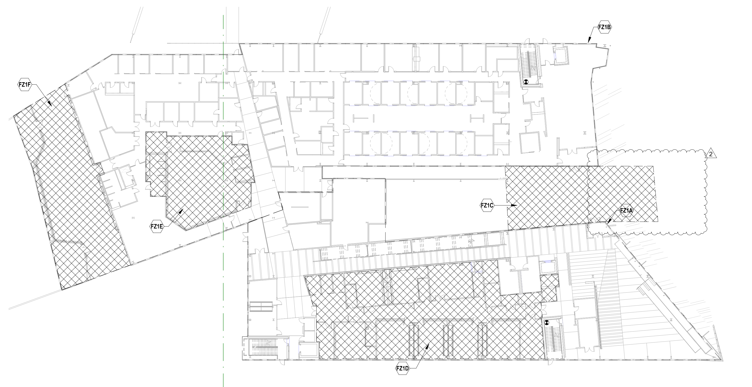
2 FIRE SPRINKLER - LEVEL 1 ZONE PLAN 1" = 30'-0"
