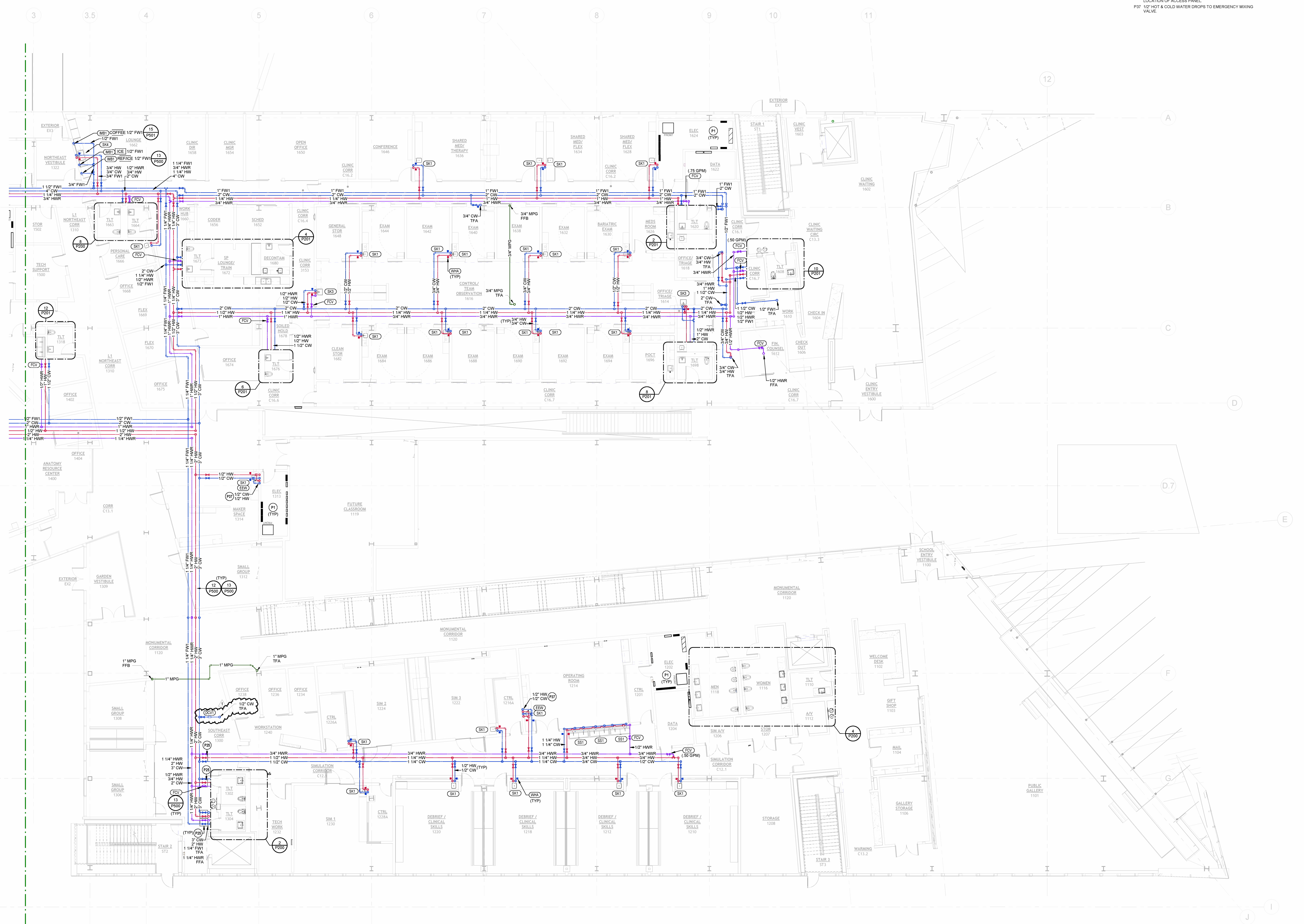
2 PLUMBING WATER & GAS - LEVEL 1 PLAN - AREA A 1/8" = 1'-0"
