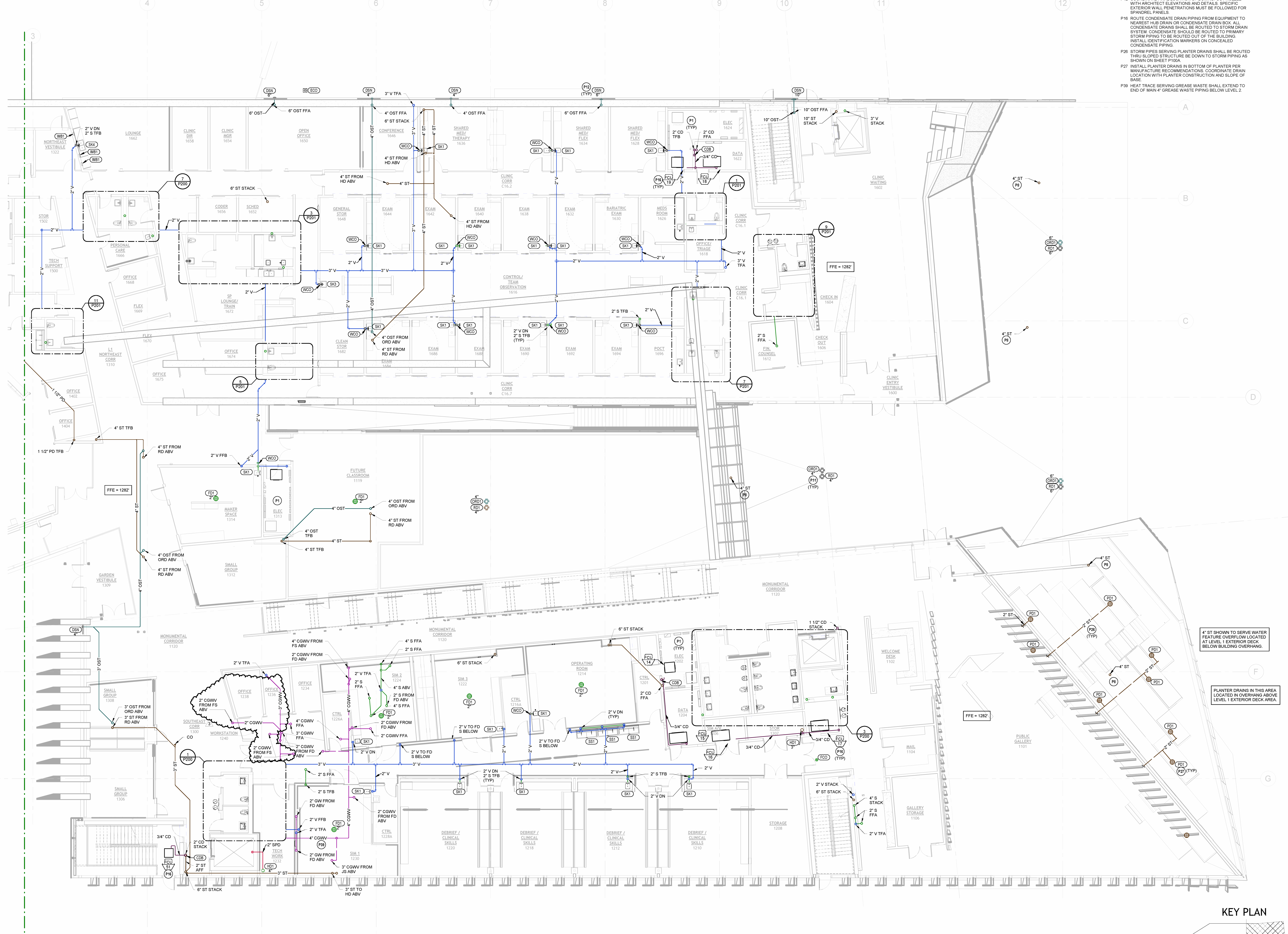
PLUMBING WASTE & VENT - LEVEL 1 PLAN - AREA A 1/8" = 1'-0"
