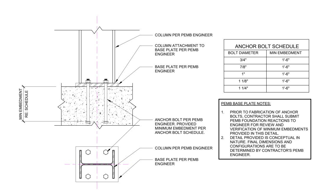
C1 TYPICAL PEMB COLUMN BASE PLATE DETAIL
