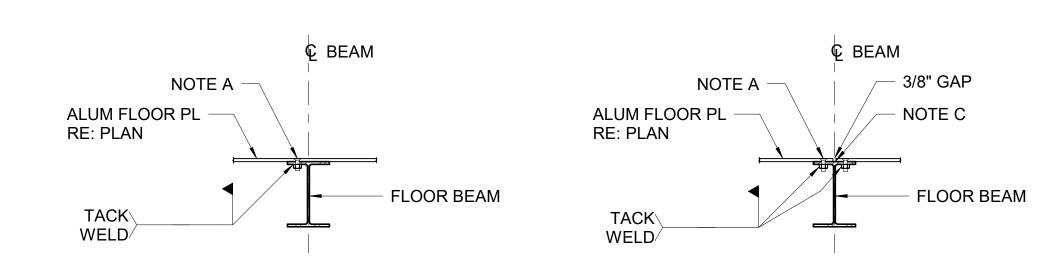
© BEAM © BEAM EDGE OF PL 3/16 2@6 – 1/4" ALUM TOE PL - NOTE D 3/16 / 2@6 ALUM FLOOR PL -RE: PLAN ALUM FLOOR PL -NOTE B - ALUM FLOOR PL NOTE A RE: PLAN RE: PLAN 3/8" GAP CENTERED
