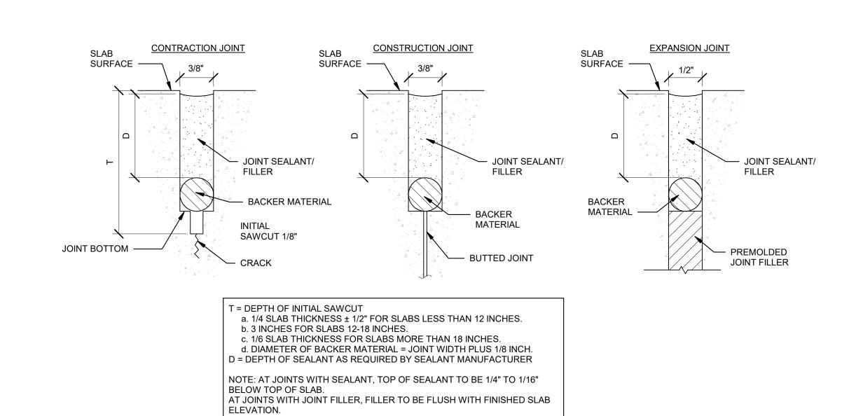
B4 TYPICAL JOINT SEALANT DETAILS AT GRADE SLABS
