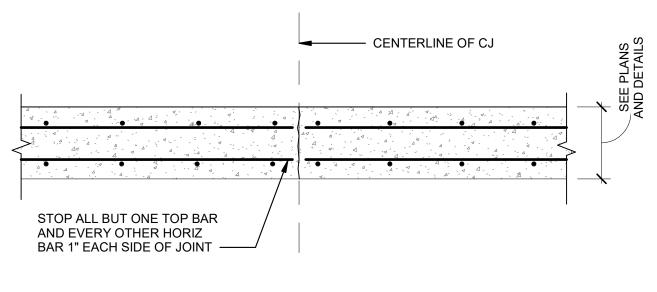
SEE FOUNDATION PLANS FOR LOCATIONS OF CONTROL JOINTS IN CONCRETE WALLS. 2-LAYERS OF REINF SHOWN. SOME WALLS HAVE ONLY ONE LAYER.
