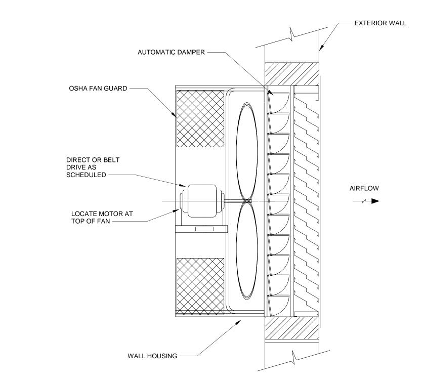
C5 WALL MOUNTED EXHAUST FAN SCALE NTS
