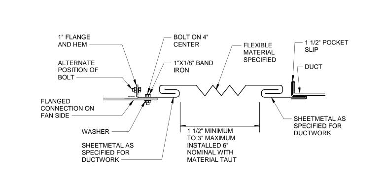
TYPICAL RECTANGULAR TO FLEXIBLE DUCT CONNECTION DETAIL
