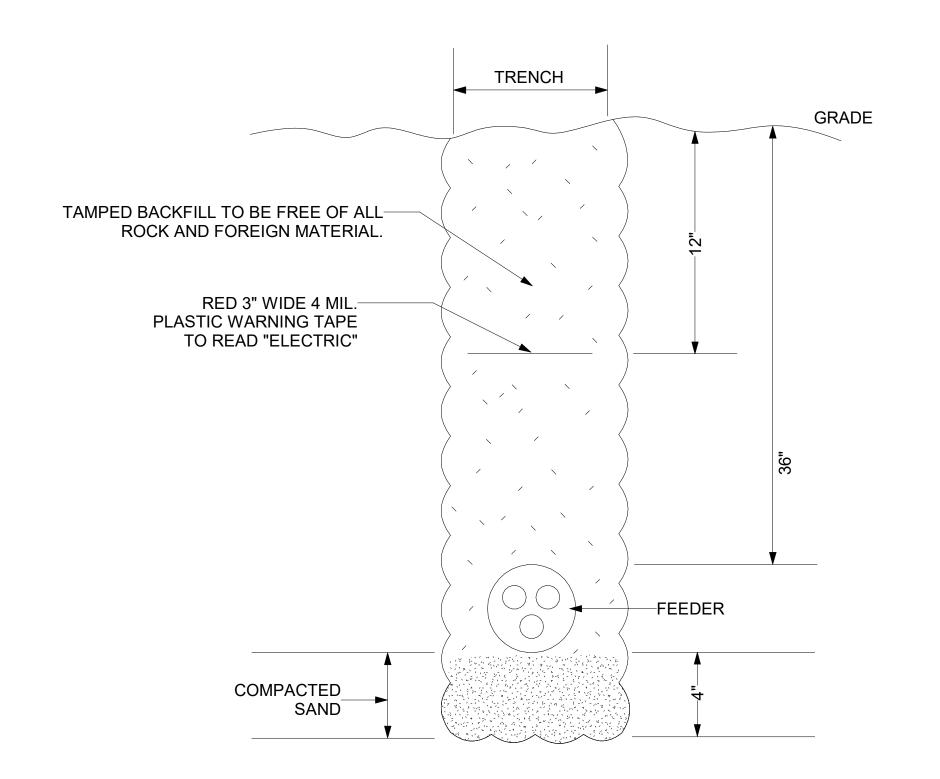
NOTE: PROVIDE SLACK CABLE AT HAND HOLES AND ENTRANCE/EXIT CONDUIT. PROVIDE SCHEDULE 80 PVC CONDUIT BELOW ROADWAYS, PARKING, AND DRIVES
