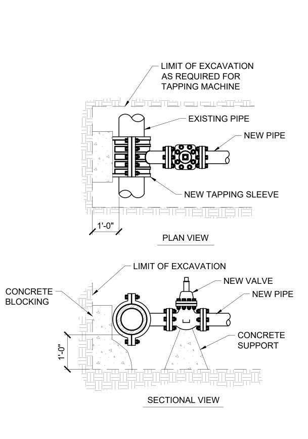
TAPPING SLEEVE AND VALVE CONNECTION SCALE N.T.S.
