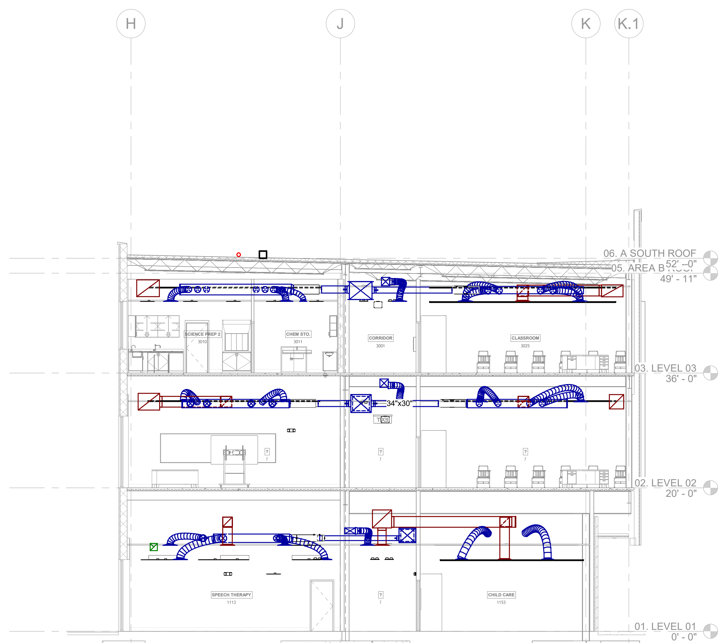
1 MECHANICAL SECTION @ A-SOUTH 1/8" = 1'-0"
